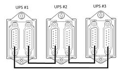
Remove the cover of 'parallel box', then connect each UPS one by one with 'parallel cable', make sure the cable is screwed to parallel port tightly.
