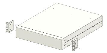
3. Slide the unit into 'rail kit' and make sure tighten the 'rack mounting screw'.
