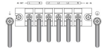
For cables well fixed, it is recommended to tie these cables to the convex of rear-panel.
